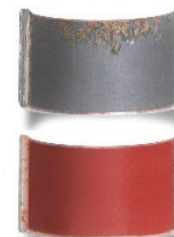
Material delamination comparison results after shock absorber rig test under 6 MPa radial load pressure and 2.6 m/s speed
