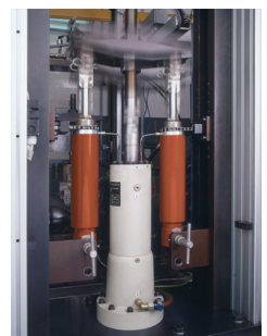
Shock absorber rig in operation at Tenneco Technology center during test of GLYCO® 298
